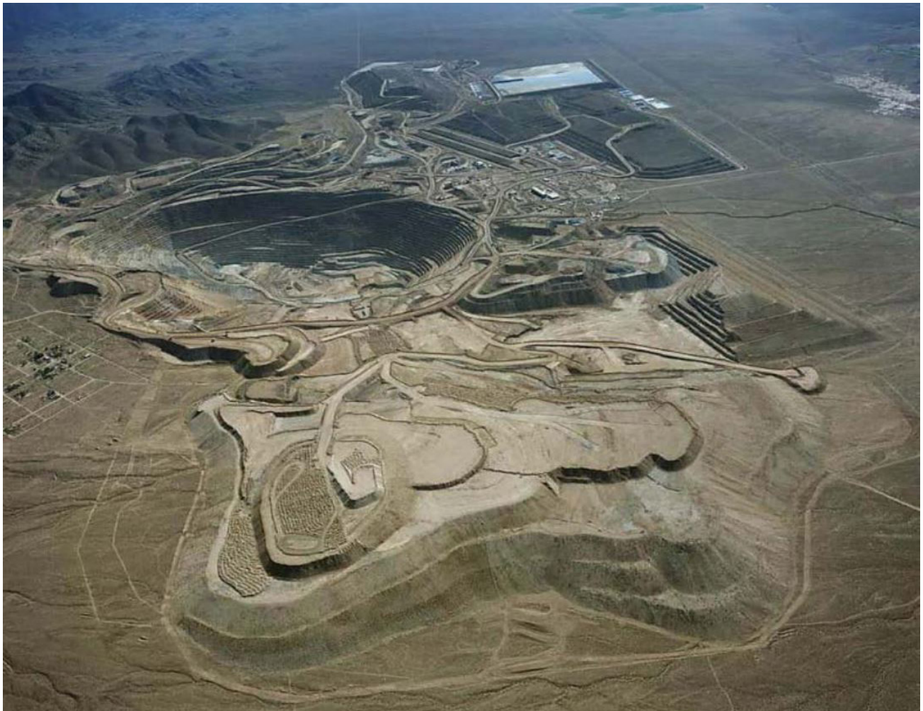
Example of open pit and heap leach mining operations: the Round Mountain Mine, Nevada, with open pit center left, waste rock dump front, and heap leach pads right and upper right 14
